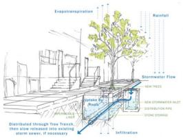
The Philadelphia Water Department's green infrastructure projects—tree trenches,rain gardens, porous paving and planters, just to name a few—are designed tostore and infiltrate stormwater runoff into the ground. By keeping this water out of our sewers, we can prevent sewer overflows that damage the health of our rivers and streams. In the last month, Hurricane Irene and Tropical Storm Lee put our green stormwater projects to the test with periods of intense rainfall.
