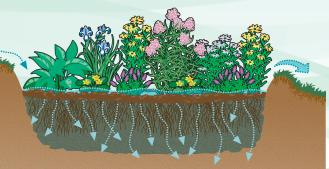
A rain garden slows the flow of rain water runoff.
